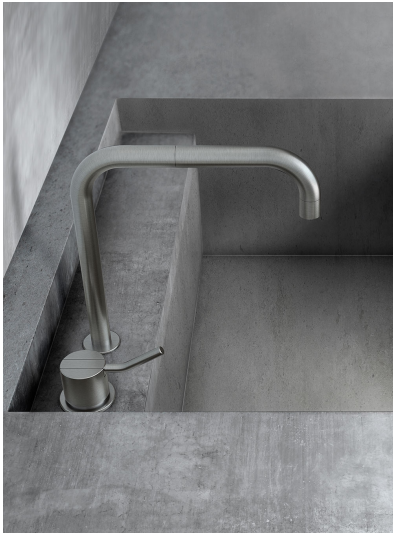
590M One-handle mixer with ceramic disc technology, with medium lever, for table mounting 500, with double swivel spout 090 with water saving aerator. Hole cut out size, mixer: 42 mm. Hole cut out size, spout: 22 mm.
